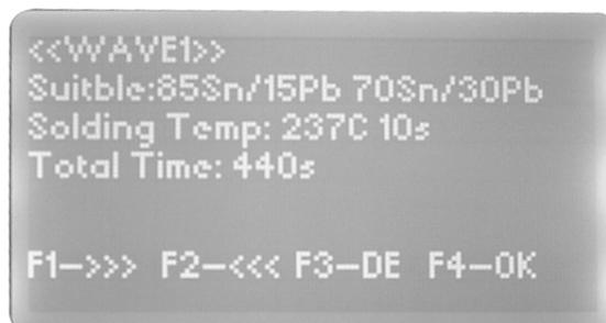
Press the “F4” button to return to the previous page, Press the temperature wave that the “F1” key carries out to make selection automatically, the process will shut down automatically upon completion and a warning buzzer will sound.
